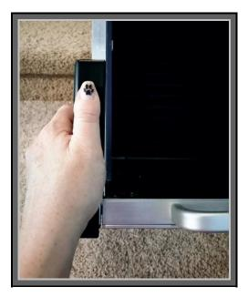
Maintain control as you push the carrier down because when the flush mount attached to the underside of the carrier gets about 2 inches away from the safety latch attached to the carriage, you will feel the gas strut release slightly and you will need to gently guide the carrier until it latches. You will hear a heavy click.
