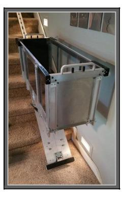
**CAUTION**: Visually inspect under the carrier to ensure that nothing is underneath it before you push it down into the loading position.
